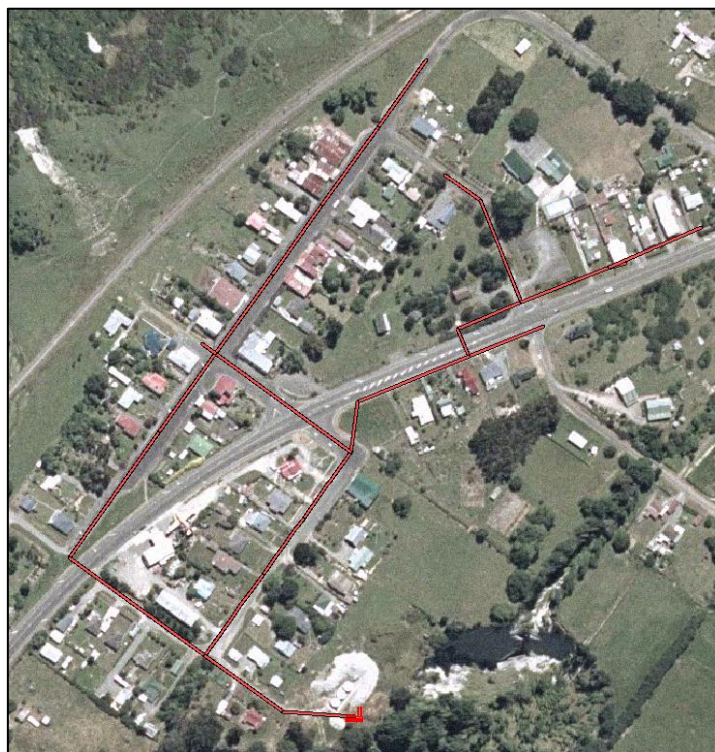
Figure 96: Extent of Mangaweka Wastewater Scheme
