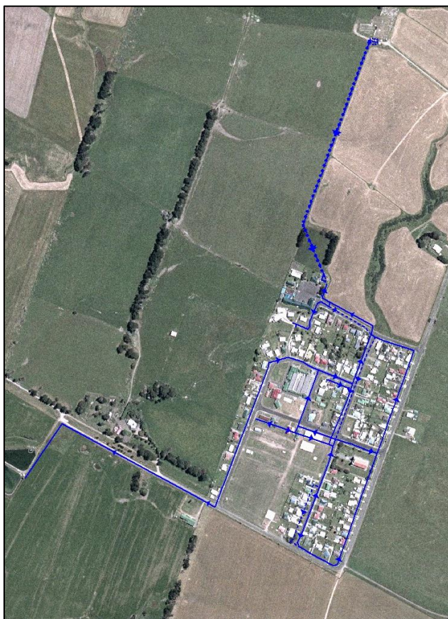
Figure 42: Extent of Ratana Water Scheme
