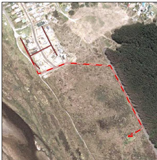
Figure 89: Extent of Koitiata Wastewater Scheme
