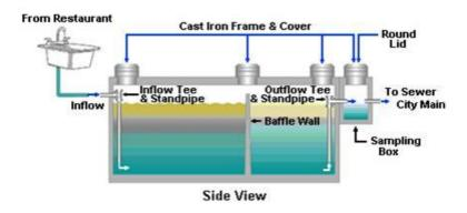
The trap has an inlet and an outlet. Baffle walls separate the unit into a number of chambers/stages. In a properly maintained grease trap, very little grease or sediment is present in the wastewater discharged to the sewer. As grease and sediment collect, the trap becomes less efficient. Grease physically interrupts the flow of liquid within and from the trap.
