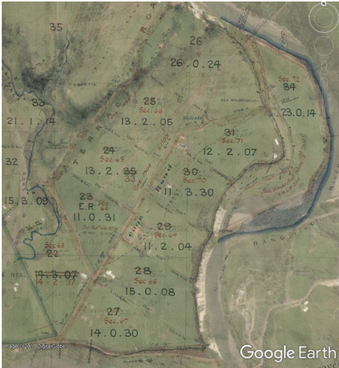
Figure 39: Google aerial with overlay of SO13796 showing the surveyed alignment of Clayton's Pack Track (T22/29) relative to Cage Road
